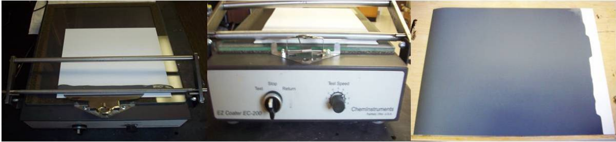
Figure 62. EZ Coater EC-200 used for the coating and production of gray samples.
