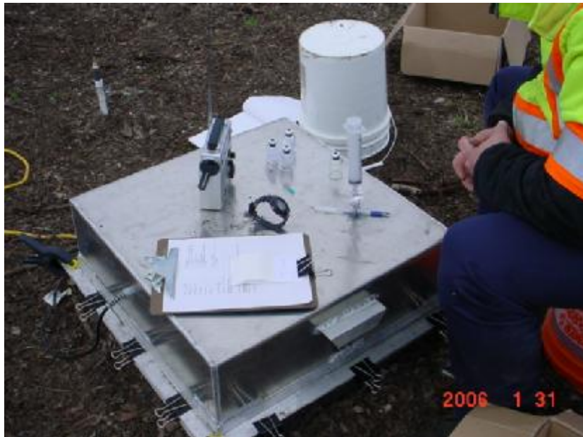
Figure 3: Static Chamber Used for Emissions Measurements
