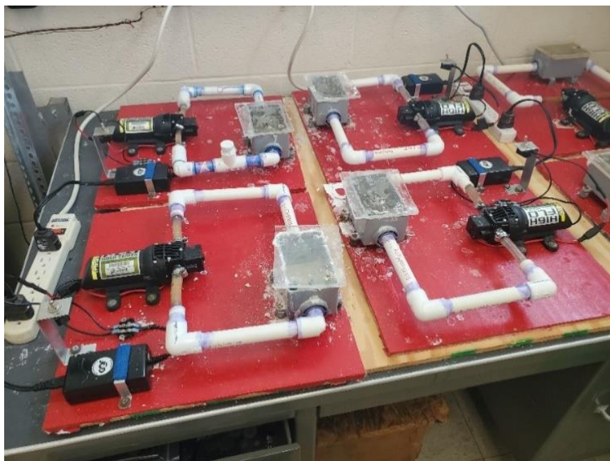
Figure 17. Four individual circulators made of a small pump connected to a sample housing by tubing.
