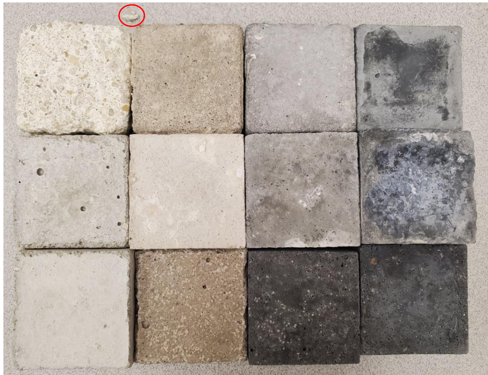
Figure 21. The eight samples after their 60 days each in the circulators compared to fresh samples. Top row - 0.7 pH. Middle row - 6.3 pH. Bottom row – fresh. Left to right - Portland, MPC Base, MPC 2020, MPC 3030.
