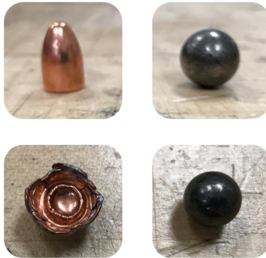
FIGURE 41. 9 MM FMJ (LEFT COLUMN) AND .50 CALIBER STEEL BALL BEARING (RIGHT COLUMN) BEFORE (TOP ROW) AND AFTER (BOTTOM ROW) IMPACTING THE TARGET.
