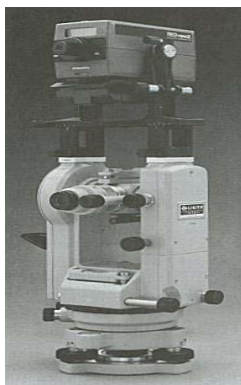
Figure 5.1 Add-On Electronic Distance Measuring Instrument Mounted on a Theodolite (Photo Courtesy of Sokkia Corporation)
