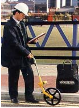
Figure 5.16 Hand Wheel (Worawat and Rasdorf 2003)
