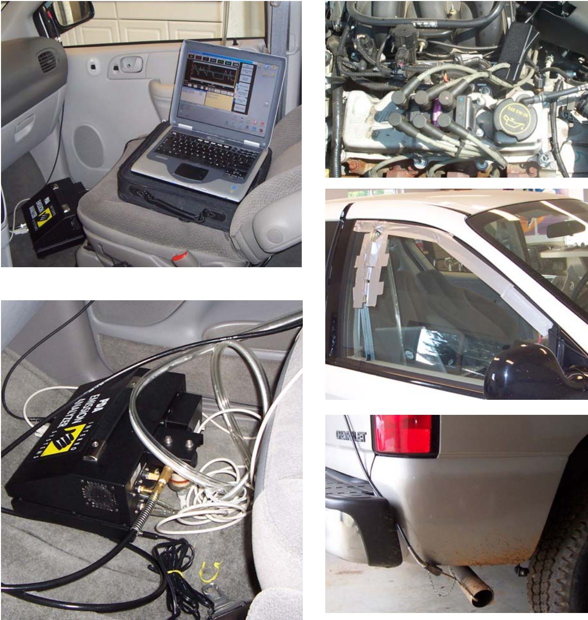
Figure 10: Emission testing set-up with 5 gas PDA analyzer and laptop interface
