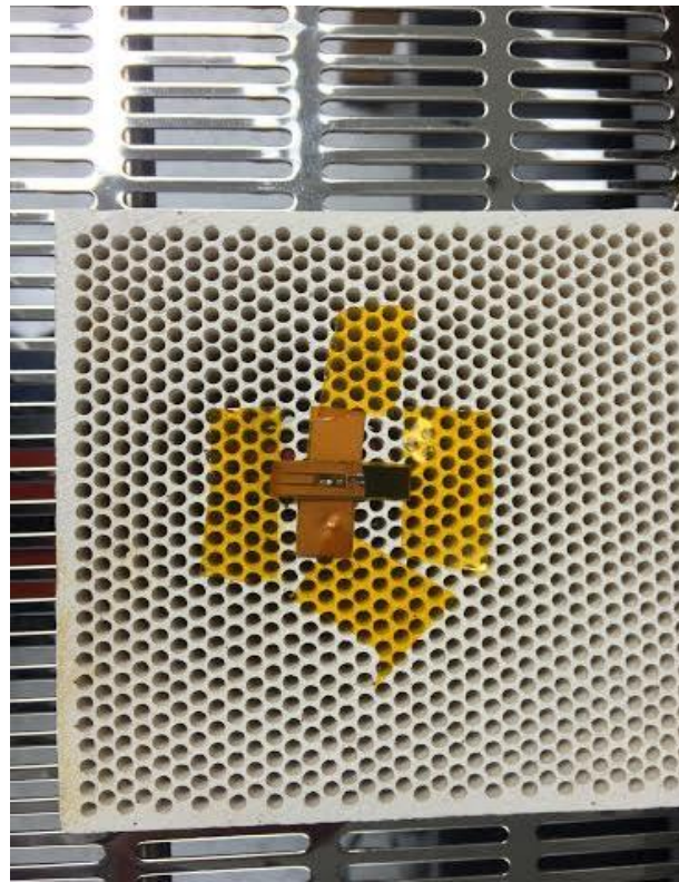
Figure 4-12 Flex module before reflow process
