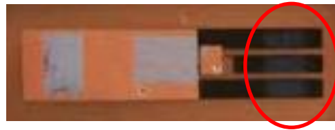
Figure 2-4 Double layer double access part
