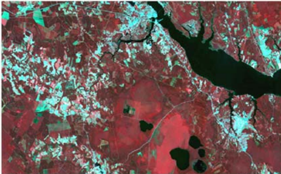
(b) The Multipsectral SPOT image with 20m spatial resolution and Albers Conical Equal Area projection.
