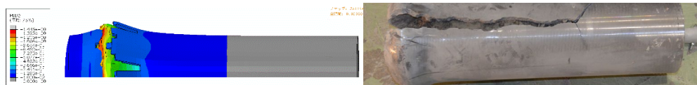
Figure 9. Comparison of Damage State of the Projectile; Experimental (Right) and Numerical (Left).
