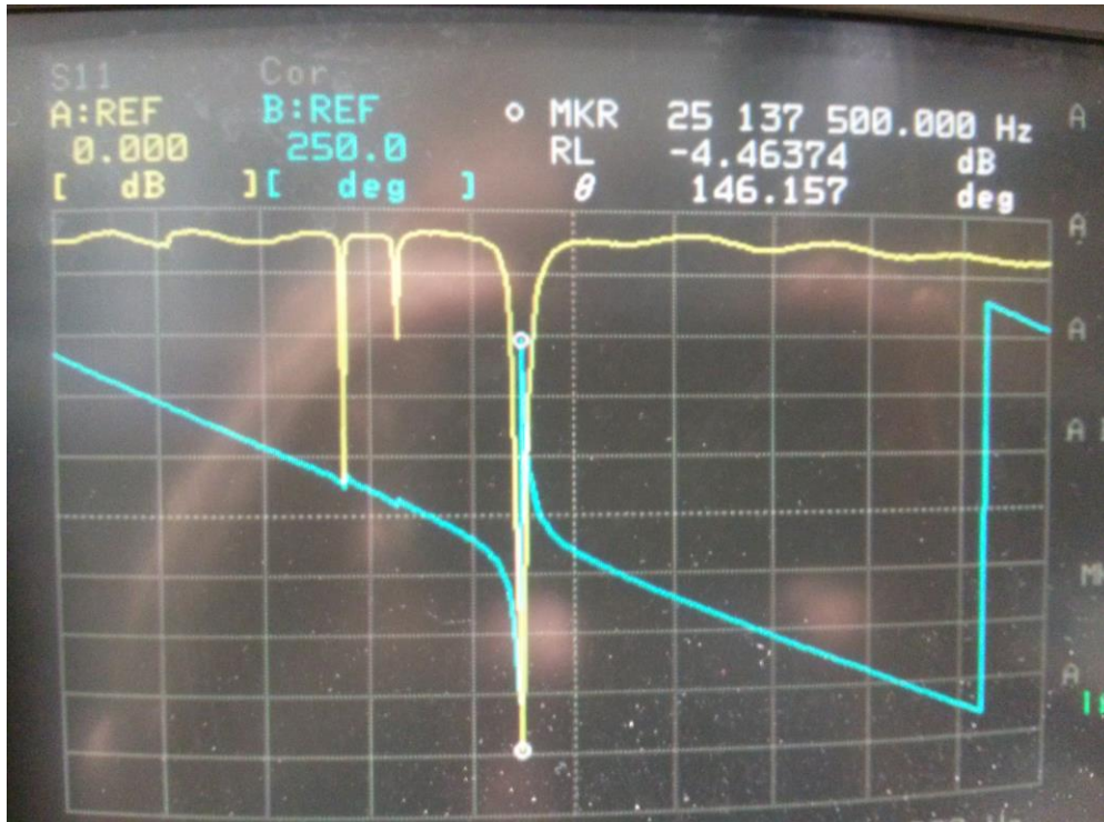
Figure 3.3 Resonance spectra of spin flipper when coupled to network analyzer inductively. These produce much weaker minima of other modes, as the primary is selected preferentially.
