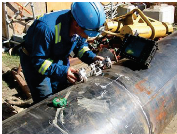
Figure 2. An illustration of an example of an NDT inspection by the phased array method
