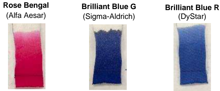
Figure 4-4. Dye solution visibility on fabric substrates with 0.6 wt% of (a) rose Bengal, (b) brilliant blue G, and brilliant blue R.
