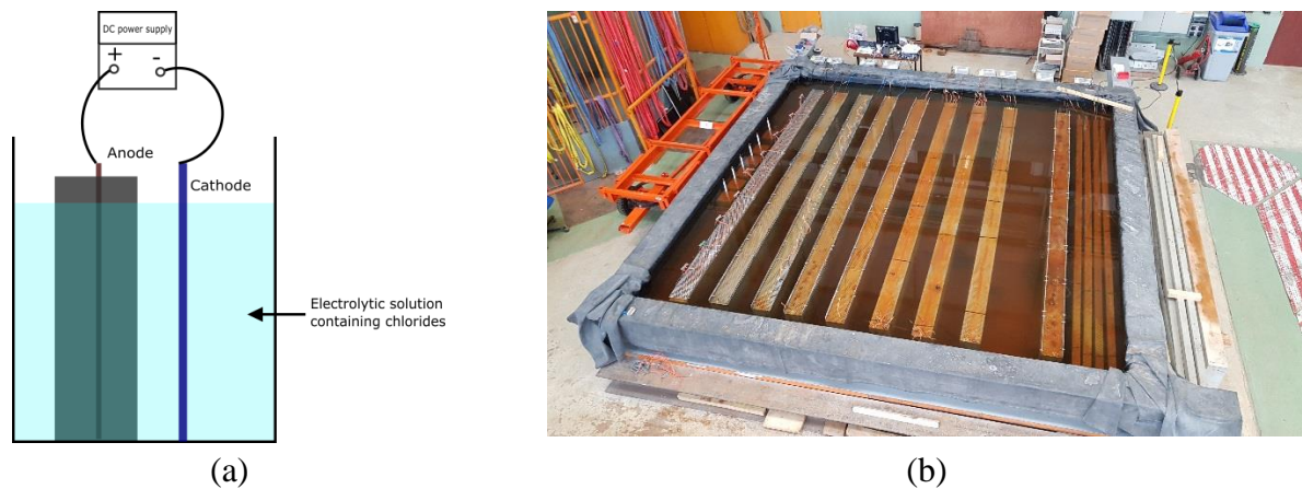
Figure 2. Accelerated corrosion technique. (a) Principle of the setup, (b) Corrosion of the campaign beams.
