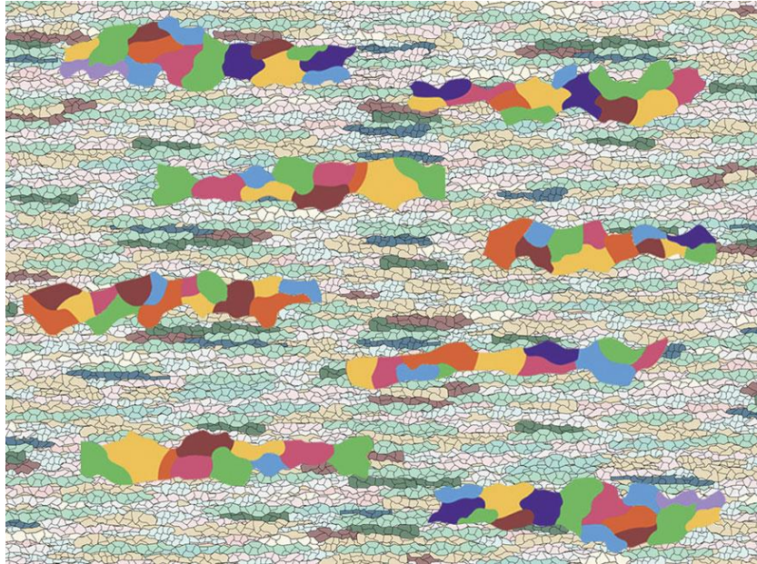
Figure 5: Schematics of an ideal lamella structure with elongated coarse grains embedded in an ultrafine-grained matrix [6].
