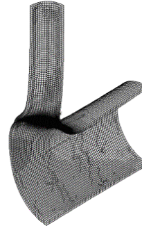
Fig. 8 Deformation and plastic zone for cylinder-nozzle model M22 at P = 28 MPa
