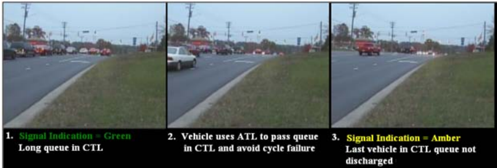
FIGURE 1-3. Example of Vehicle Using ATL during Green to Clear the Intersection
