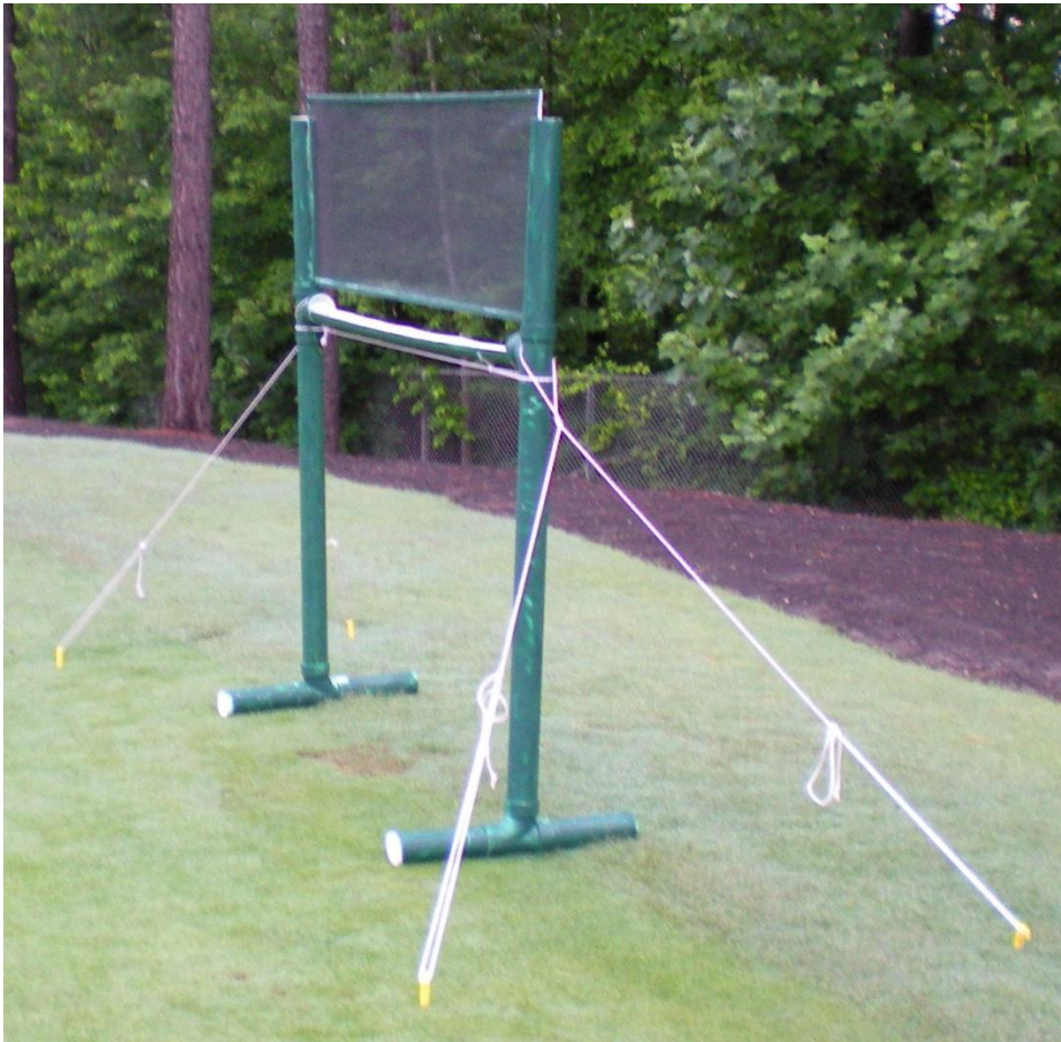
Figure 2. Flight intercept trap 1.2 m – 1.8 m above the ground.
