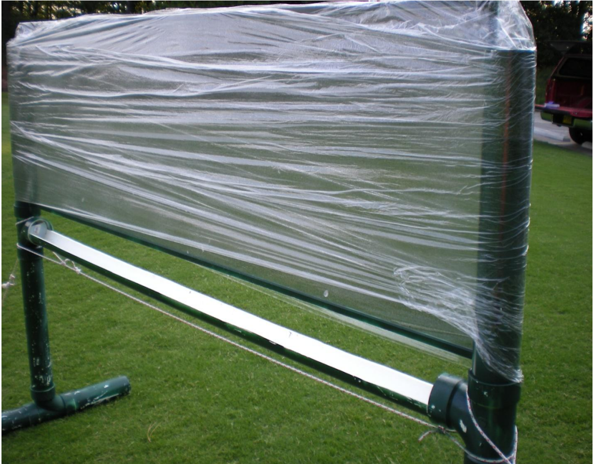
Figure 4. A 0.6 m – 1.2 m flight intercept trap wrapped in plastic wrap and sprayed with Tanglefoot®.
