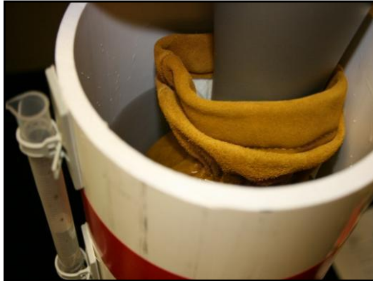
Figure 3.5 Whole Glove Bulk Measurement
