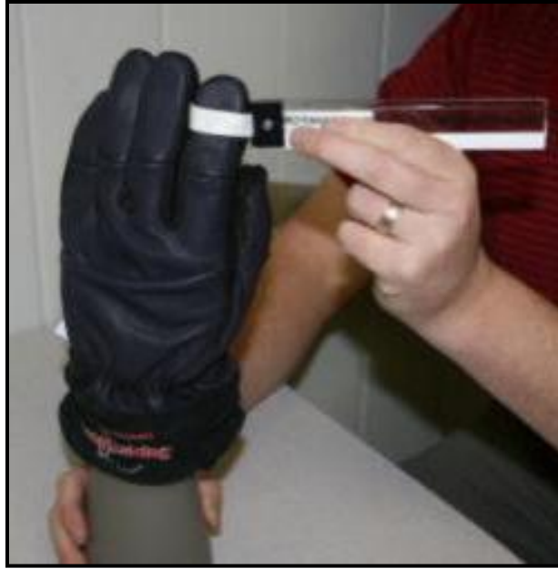
Figure 3.6 Measurement of Index Finger Circumference
