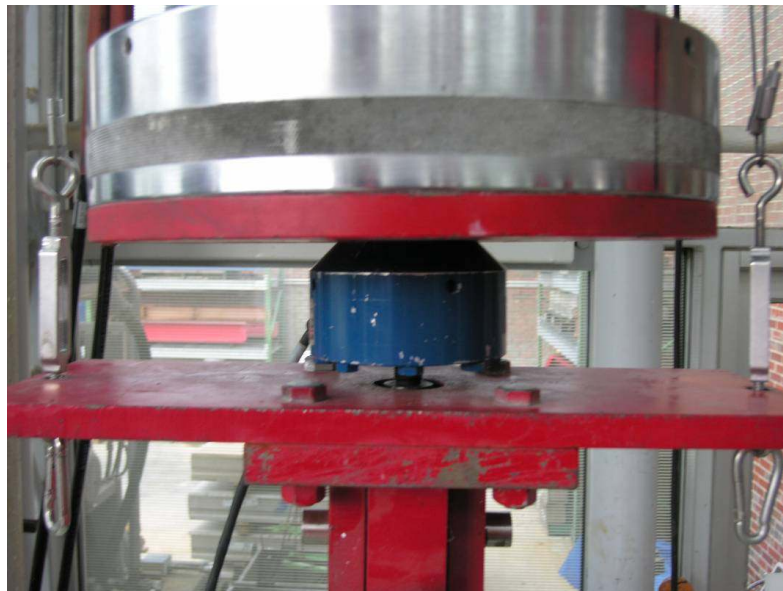
Figure 3.12 Fatigue Test Load Cell Setup
