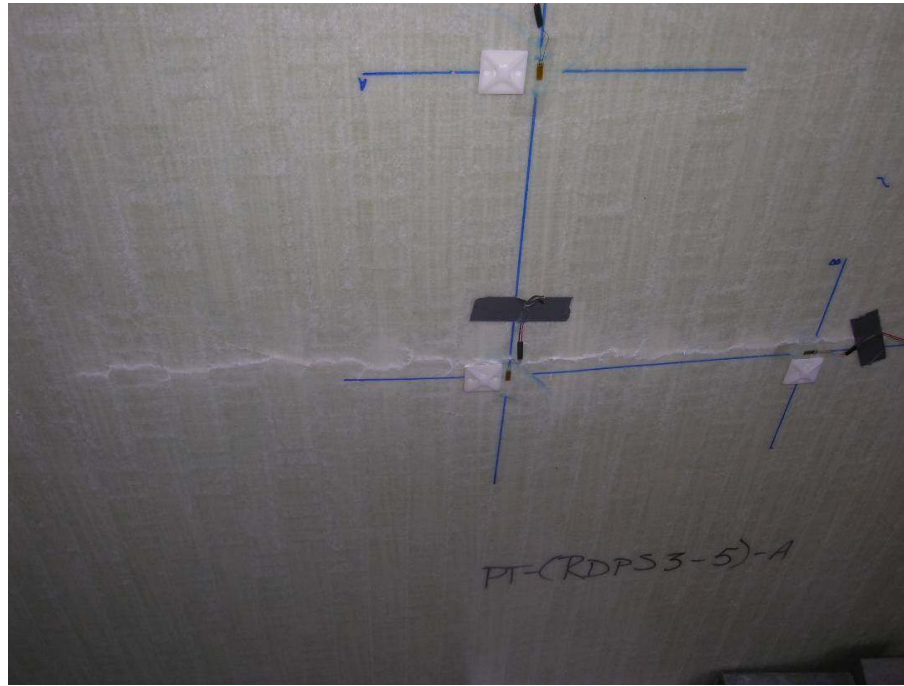
Figure 4.5 Tension Rupture of Skin
