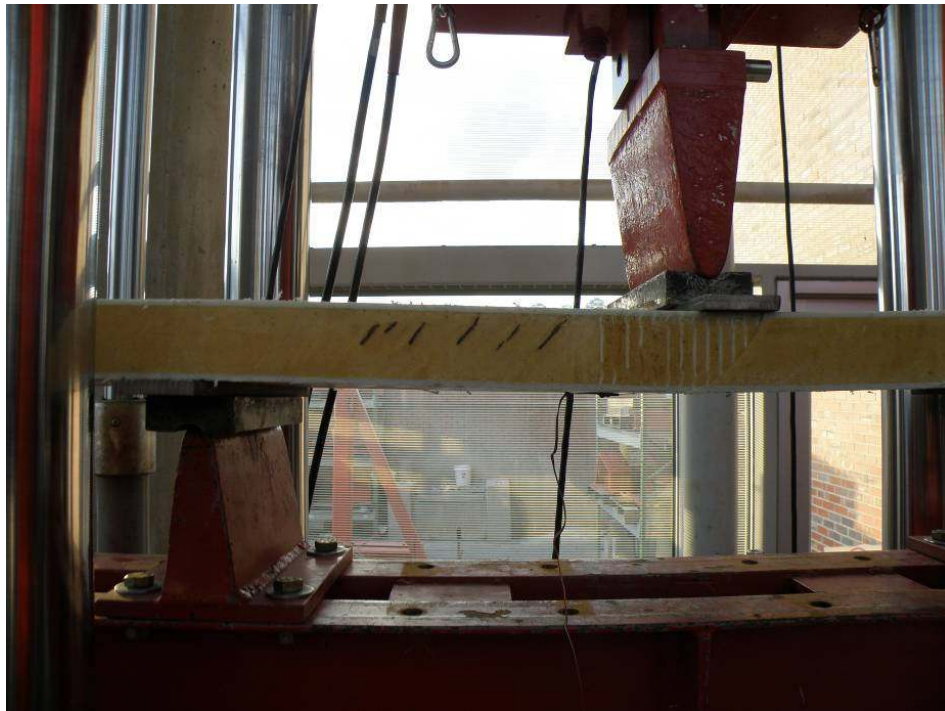
Figure 5.5 Cracking first noticed at 6000 cycles
