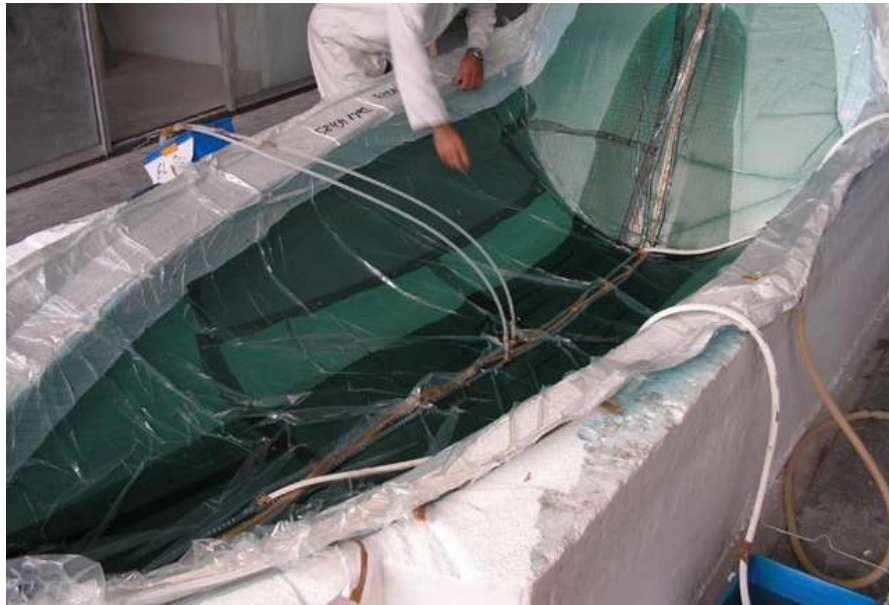
Figure 2.2 Fusion of the FRP skin of a boat hull
