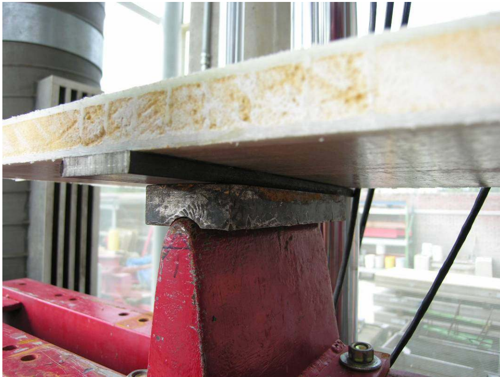
Figure 3.8 Fatigue Testing Supports
