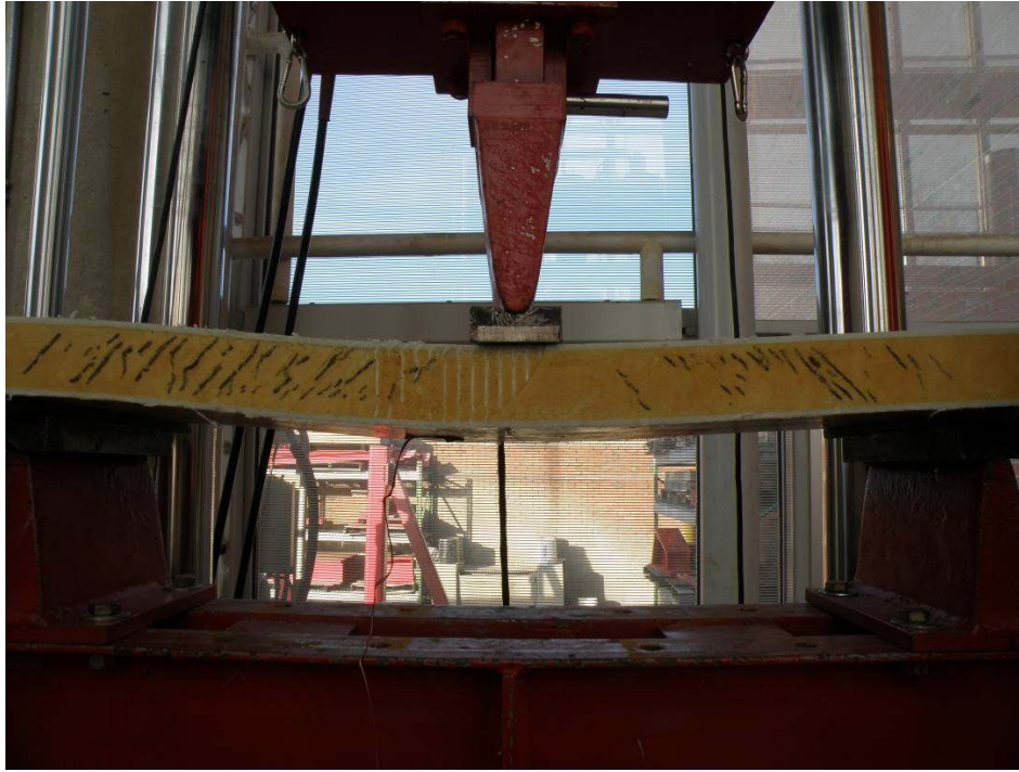
Figure 5.7 Cracking at 240,000 cycles
