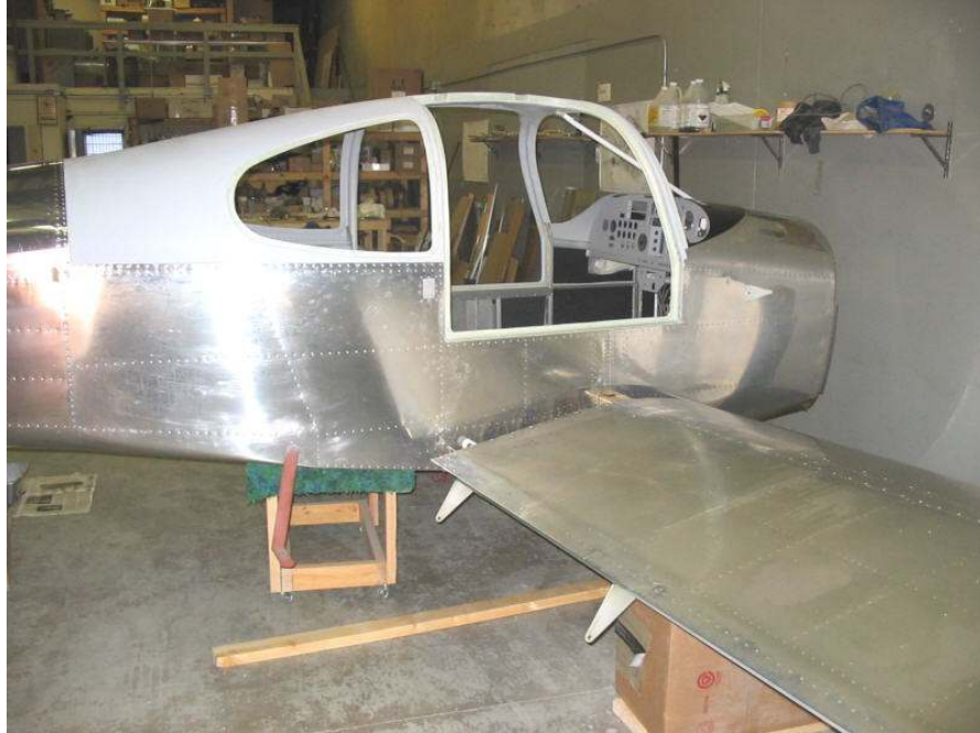
Figure 2.1 Outer shell of airplane made from aluminum sandwich panels
