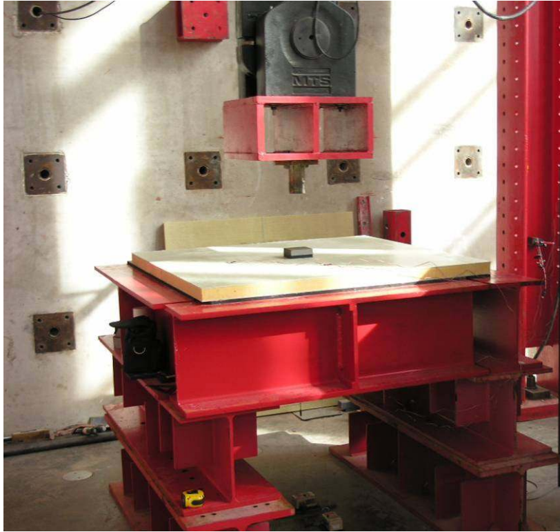
Figure 3.4 Two-Way Bending Supports
