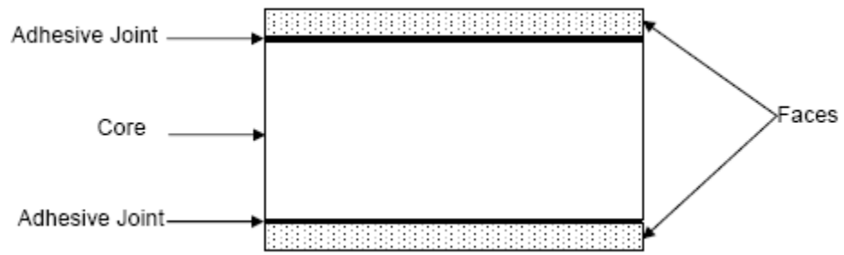
Figure 2.5 Sandwich Panel Components
