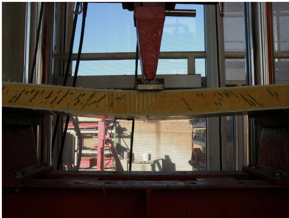
Figure 5.6 Cracking at 150,000 cycles
