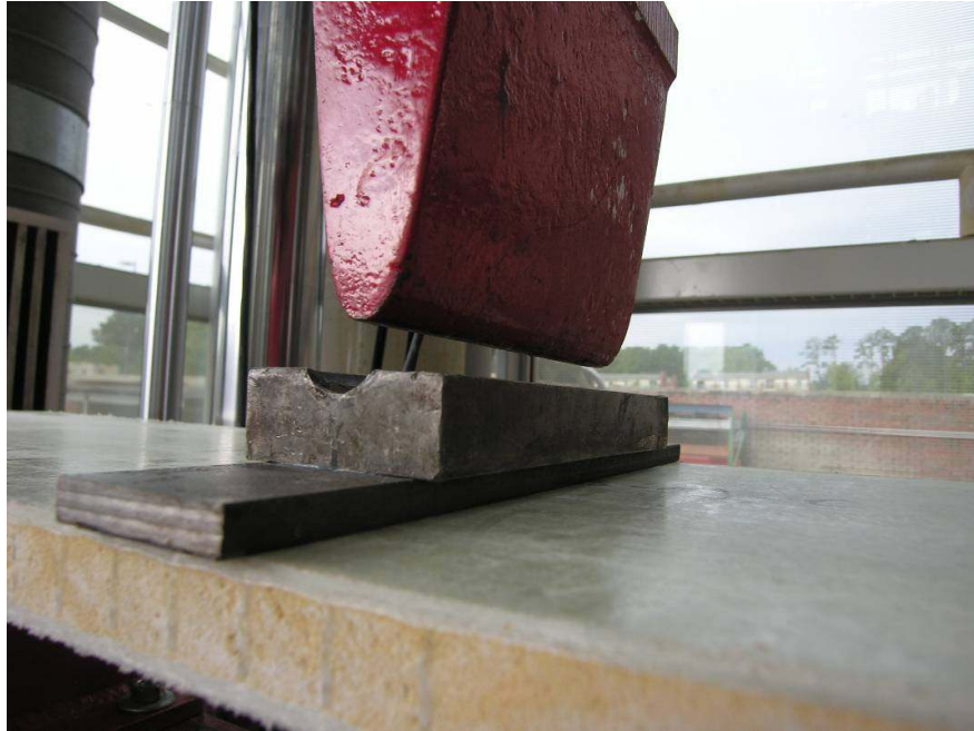
Figure 3.9 Loading Plate at Mid-Span
