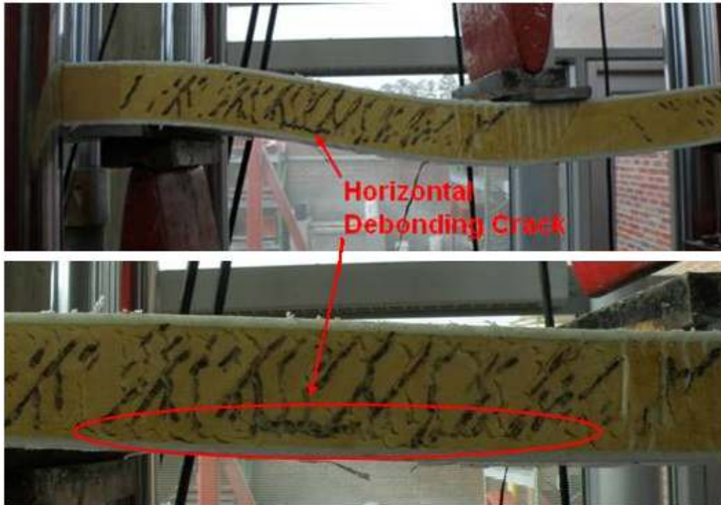
Figure 5.8 Cracking at 300,000 cycles
