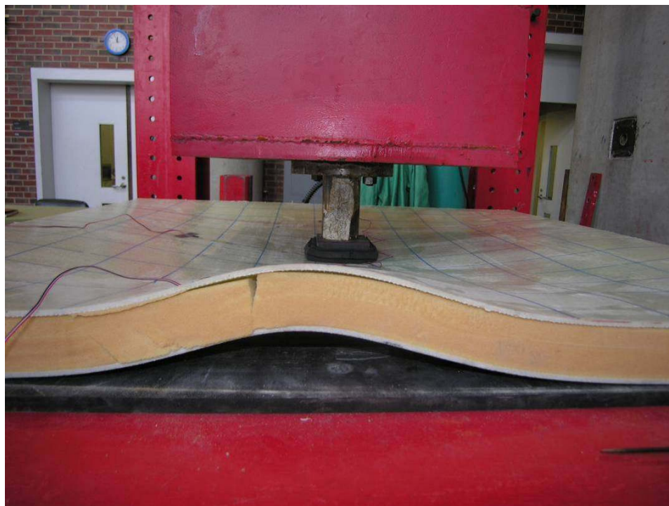
Figure 4.4 Delamination between foam and skin layers
