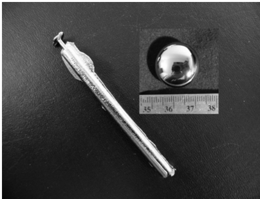
Figure 1.1 Zr- based BMG button and ingot prepared by arc melting and drop casting in inert gas atmosphere
