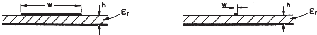
Figure 3.6: Microstrip Lines: (a) Very wide ( w \gg h ) and (b) Very Narrow ( w \ll h ) lines. Taken from Edwards and Steer [11].
