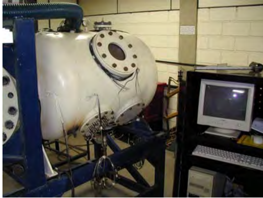
FIGURE 3.1 – Pressure Vessel manufactured for simulating underwater wet welding up to 100 meters of water column
