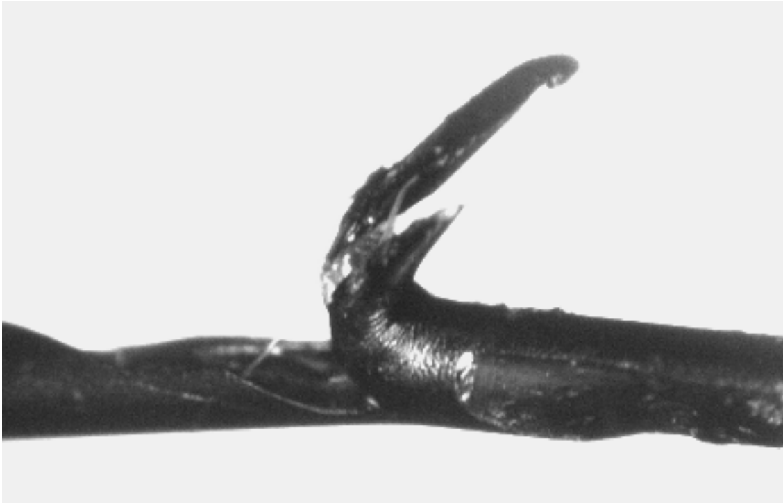
Figure 4. 34: Barb deformed at the place of maximum stress.
