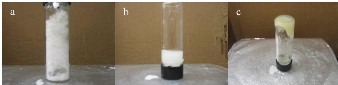
Figure 7.2 “Click”-precursors mixed together (CNC-PR and CNC-AZ) (a), “Click”-precursors after an addition of water (b) and gel formation after adding the catalysts, copper sulfate and ascorbic acid (c).
