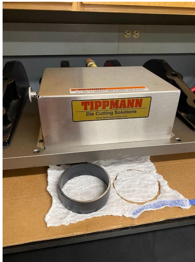
Figure 3.2: Die cutting the samples to create test specimens.
