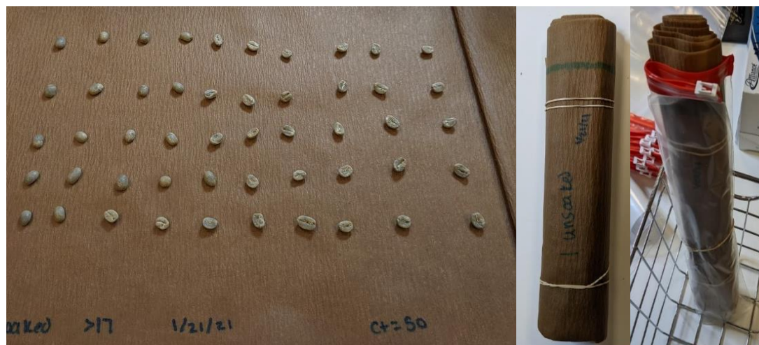
Figure I.2 Green Coffee Beans on Germination Paper (left), Wrapped Up (middle), and Wrapped in Plastic Bags to Retain Moisture During Incubation (right).
