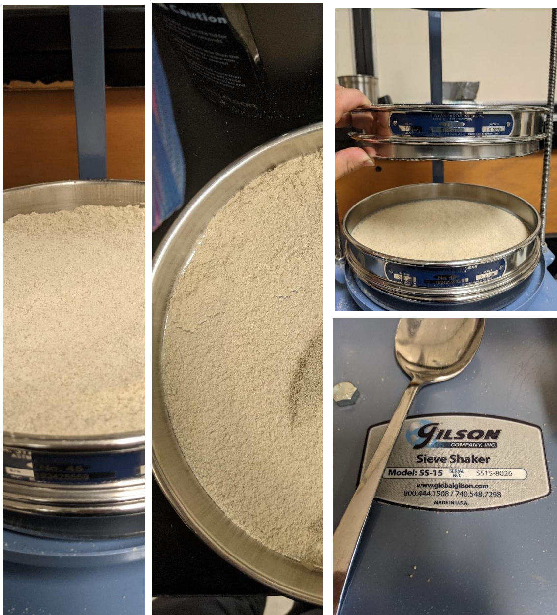
Figure F.3 Ground Green Coffee Separated by Particle Size Using a Sieve Shaker.
