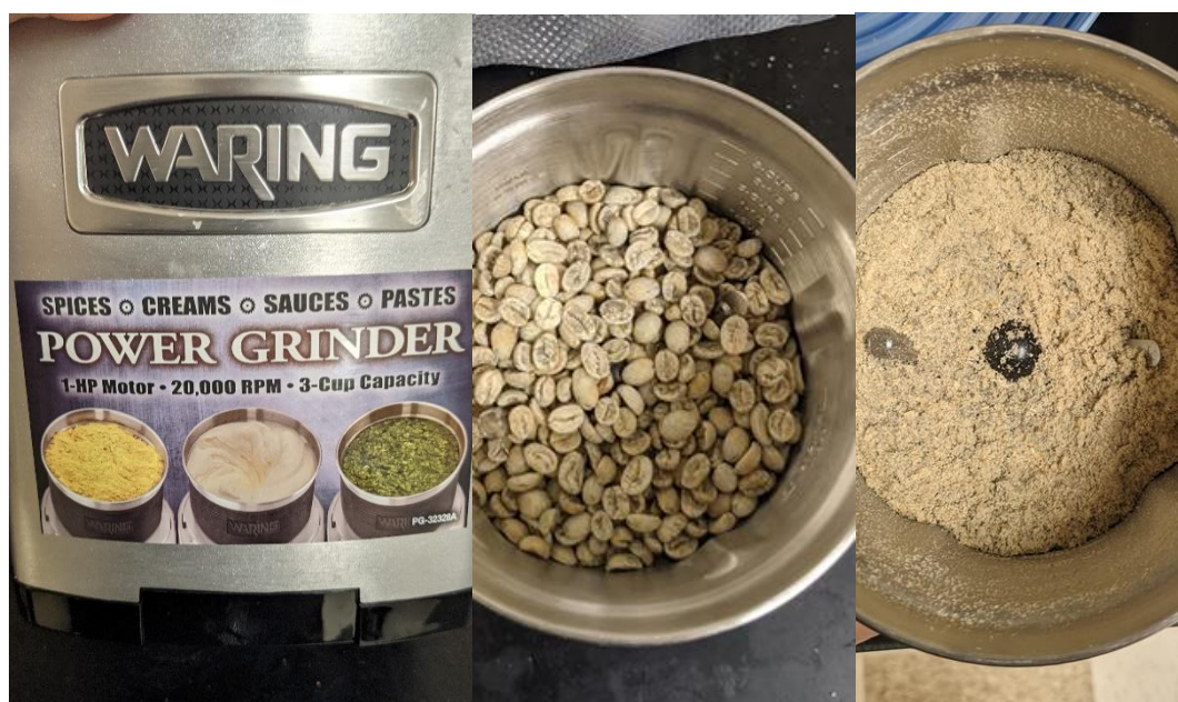
Figure F.1 Grinder (left), Frozen Green Coffee Beans (middle), and Green Coffee Beans After Grinding for One 30-Second Interval (right).
