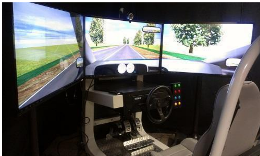
Figure 2: The STISIM Drive 3 Console simulator used in this experiment.
