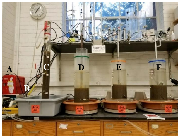
Figure 06. Experimental setup showing a) refrigerated influent, b) inline mixers, c) SBR, d) CTB1 with lower average total shear to SBR, e) CTB2 with equal average total shear to SBR, f) CTB3 with higher average total shear to SBR
