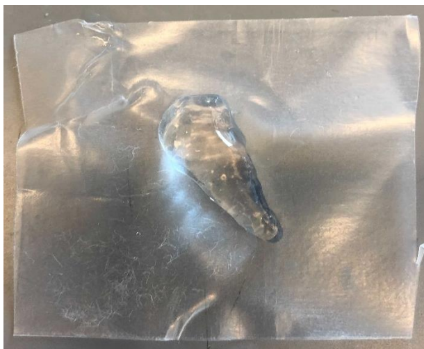
Figure 3.5. A picture of the t-BCN gels containing erlotinib prodrug and 24 hours of gelation.
