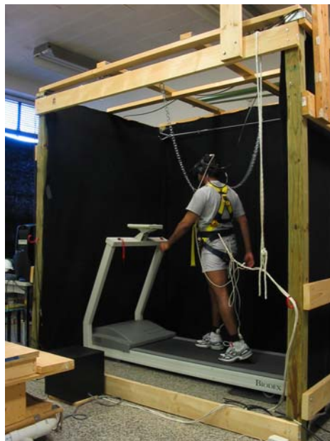
Figure 9.2 Canopy structure with safety harness suspension system and treadmill.
