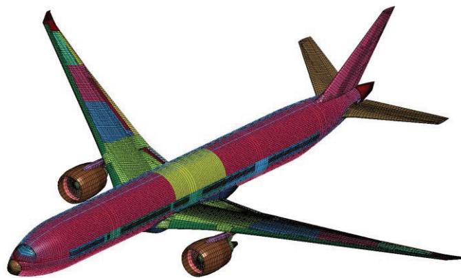
Figure 1. Finite Element model of B777
