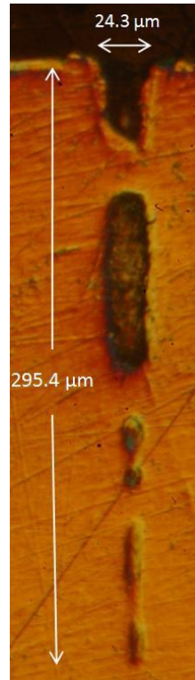
Hole Produced by 10 Pulses from the Analog Circuit
