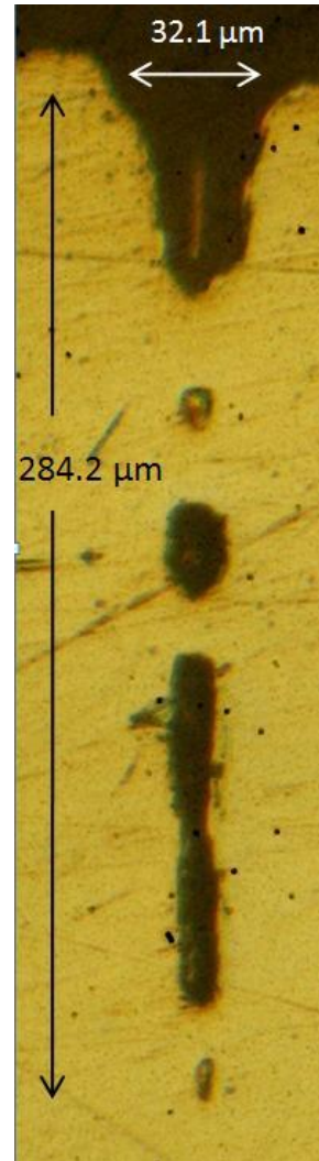
Hole Produced by 10 Pulse Analog Circuit at 16.1 kHz
