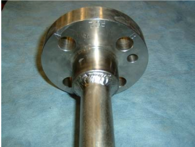
Figure 2.1 Socket-welded piping specimen
