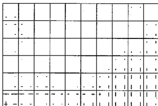
Figure 10: Crushed area at failure
