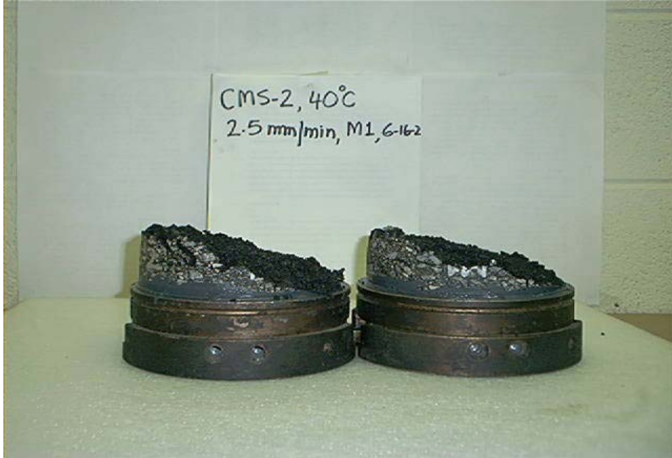
Figure 8-9 Shear failure of CMS-2 specimen (m1 6-16-2) at 1.0mm/min, 40 °C
