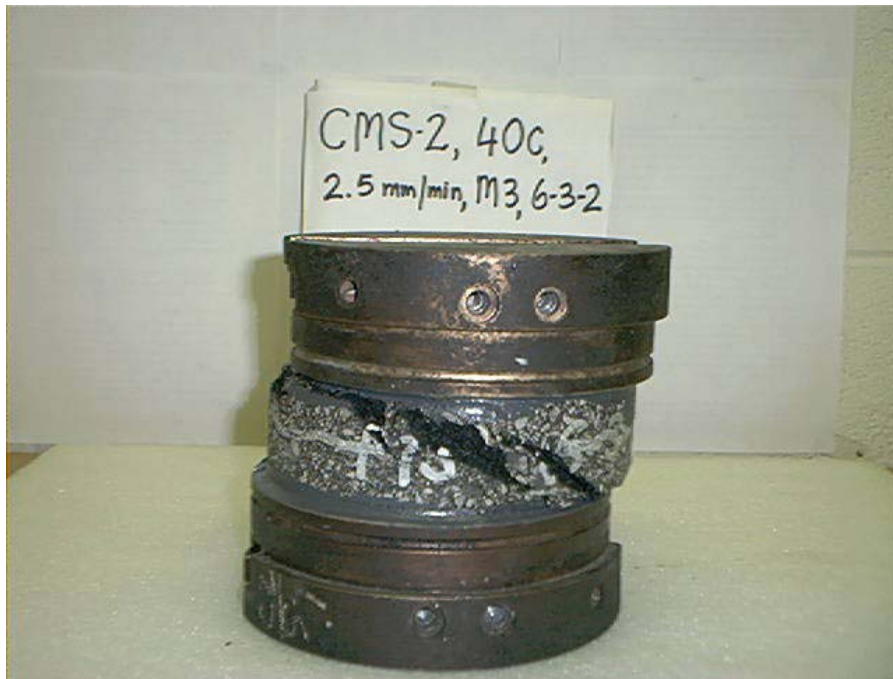
Figure 8-10 Shear failure of CMS-2 specimen (m3 6-3-2) at 1.0mm/min, 40 °C
