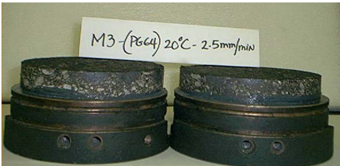
Figure 8-14 Shear failure of PG64-22 specimen (25mm3) at 2.5 mm/min, 20 °C
