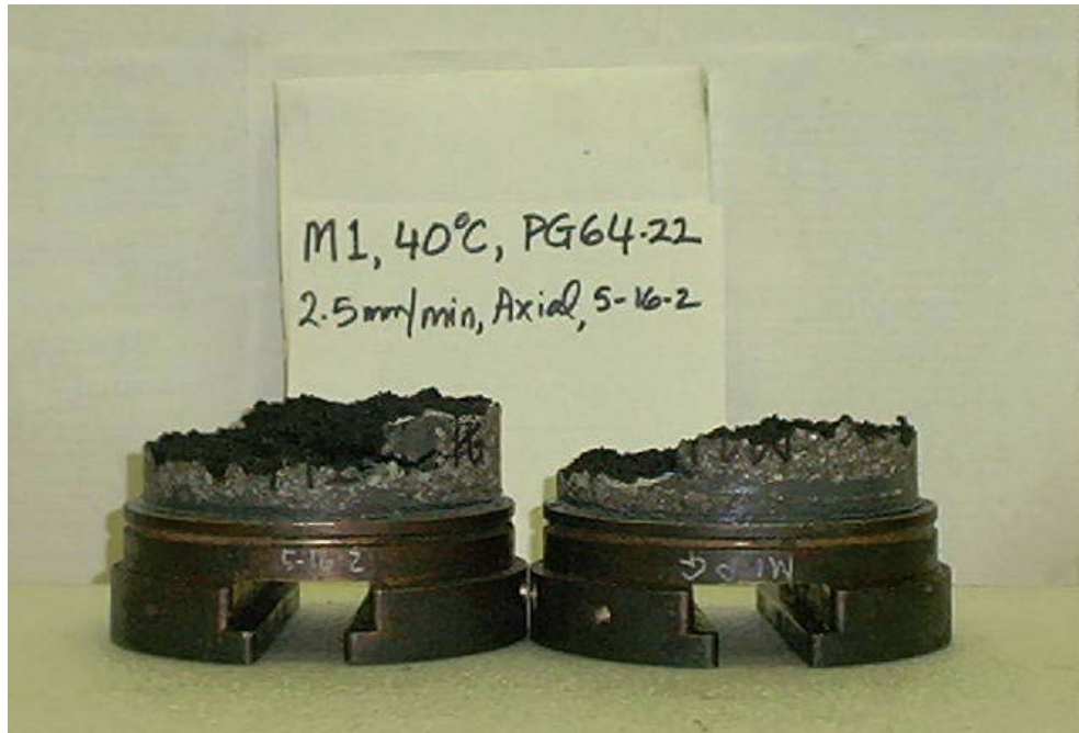
Figure 8-5 Axial failure of PG64-22 specimen (M1 5-16-2) at 2.5 mm/min, 40 °C
