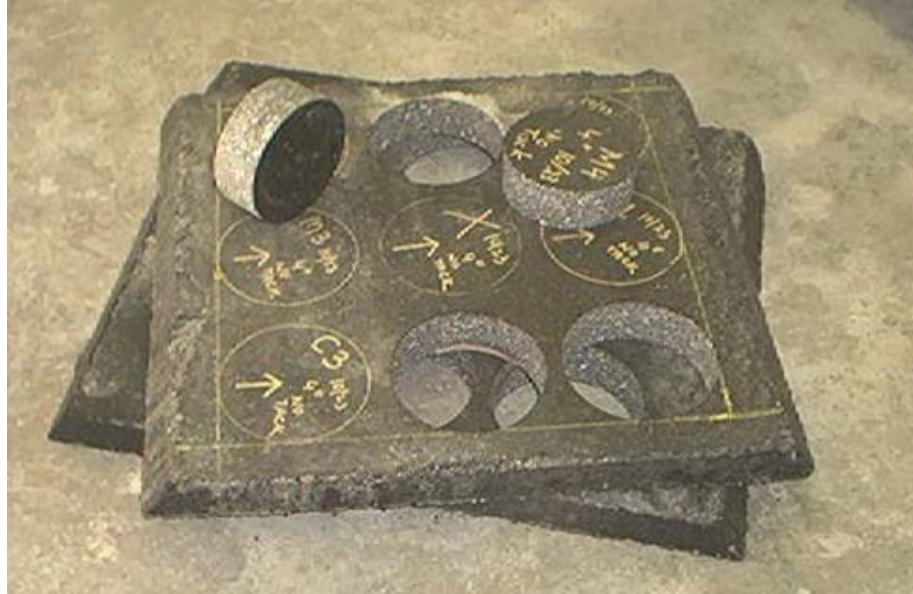
Figure 8-1 Debonded composite AC-AC slab without tack coat
