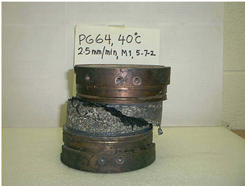
Figure 8-12 Shear failure of PG64-22 specimen (m1 5-7-2) at 2.5 mm/min, 40 °C
