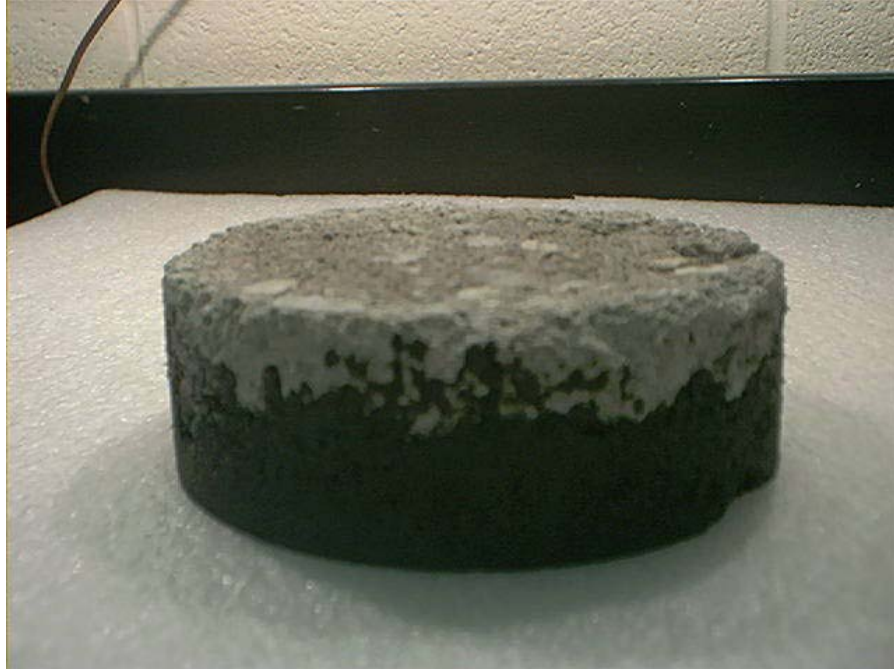
Figure 8-23 Composite CTB-AC specimen
