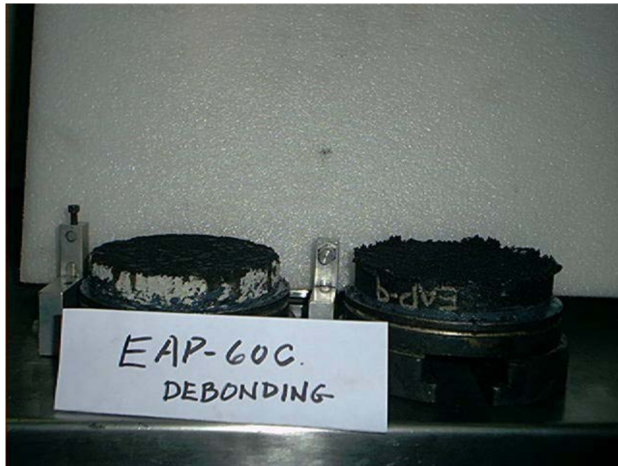
Figure 8-30 Debonded CTB-AC specimen primed with EA-P, 60 °C
