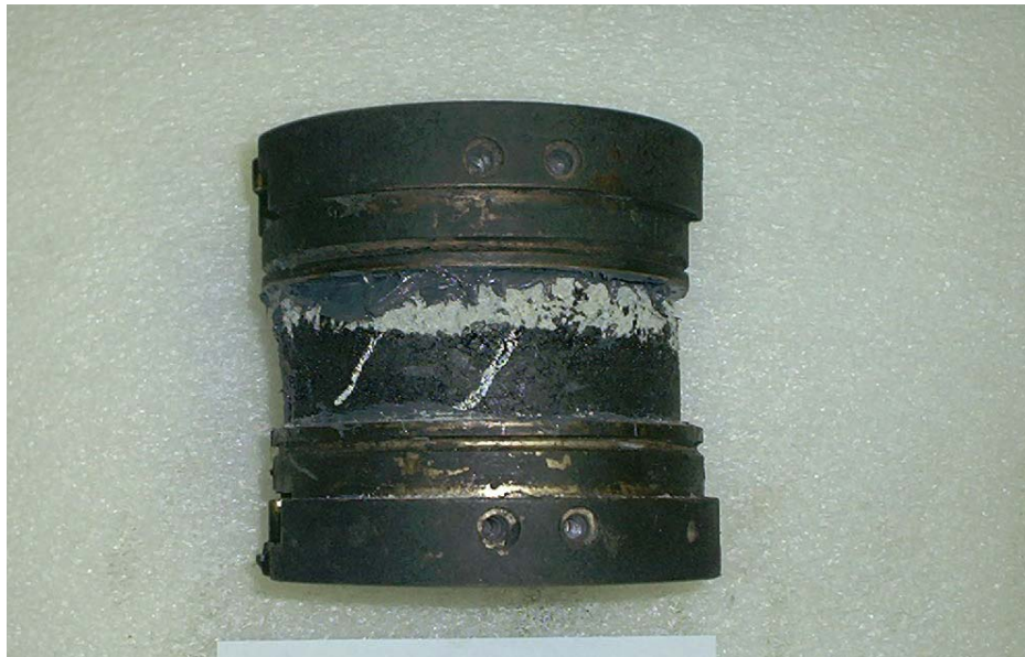
Figure 8-28 CTB-AC specimen primed with CSS-1h, sheared at 1mm/min (40 °C)
