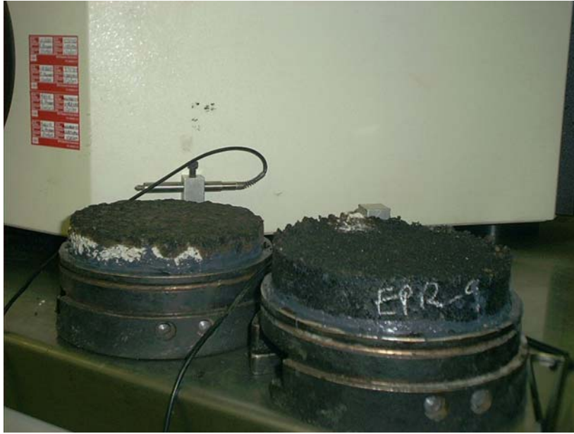
Figure 8-29 CTB-AC specimen primed with EPR-1, sheared at 1mm/min (60 °C)
