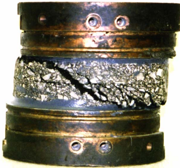
Figure 8-11 Shear failure of CMS-2 specimen (c1 6-3-2) at 2.5mm/min, 40 °C
