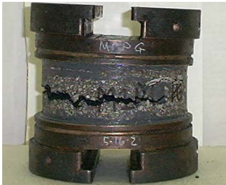
Figure 8-4 Axial failure of PG64-22 specimen (M1 5-16-2) at 2.5 mm/min, 40 °C
