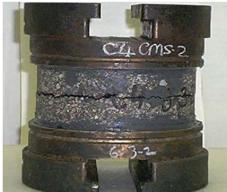
Figure 8-2 Axial failure of CMS-2 specimen (C4 6-3-2) at 2.5 mm/min, 40 °C
