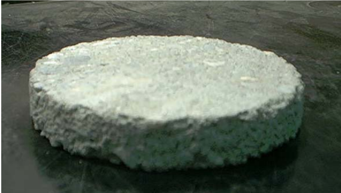
Figure 6-5 Photo of a 1-inch thick CTB 'disk'
