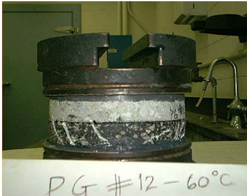
Figure 8-20 PCC-AC specimen tacked with PG64-22 (cracks highlighted in white)
