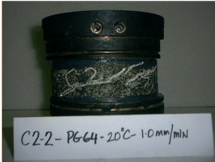
Figure 8-13 Shear failure of PG64-22 specimen (1mmc2_1) at 1.0 mm/min, 20 °C
