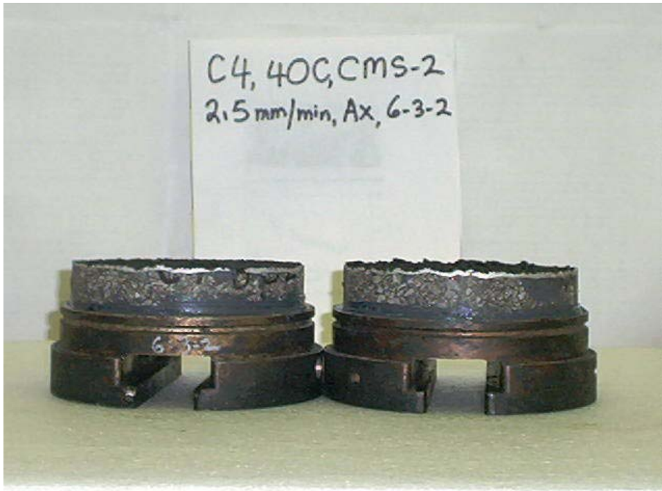
Figure 8-3 Axial failure of CMS-2 specimen (C4 6-3-2) at 2.5 mm/min, 40 °C
