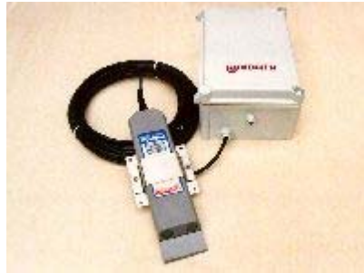
Figure 5 . Starflow ultrasonic Doppler flowmeter used to measure water velocity and depth at the outlet of subwatershed T4.
