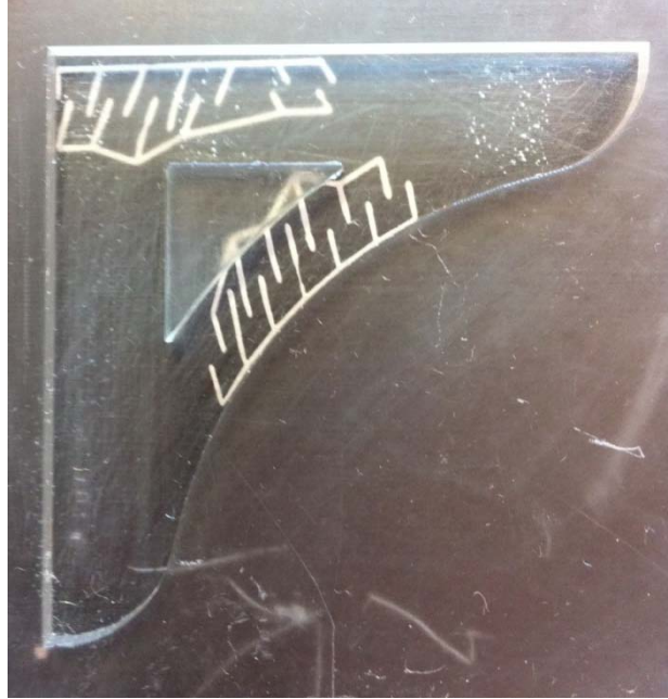
Figure 35 Electrode network printed by nScript Microdispensing machine
