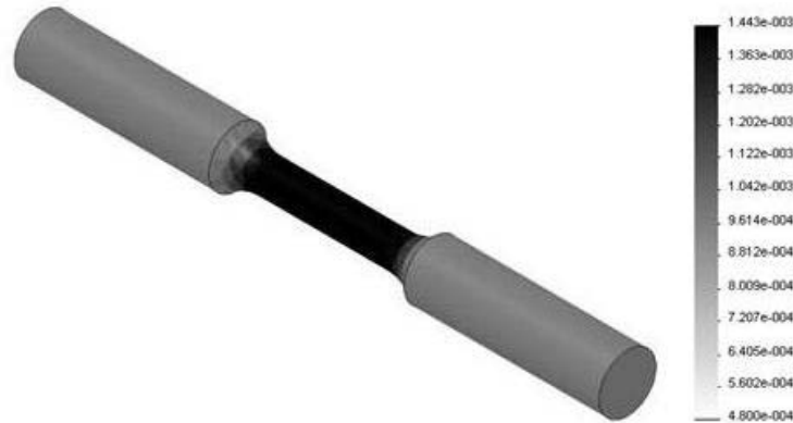
Figure 17 Equivalent strain plot of a cylindrical tensile specimen under an axial load
