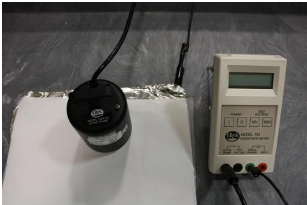
Figure 3.93.7: TRek model 152 resistivity meter and TRek model 152-CR probe set up
