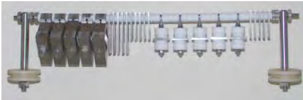
Fig.4 Corrosion monitoring system for the water-shielding tank
