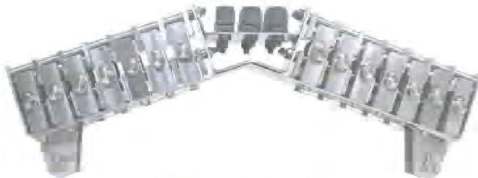
Fig. 3 Set of samples prepared from primary collector bolts in the holder
