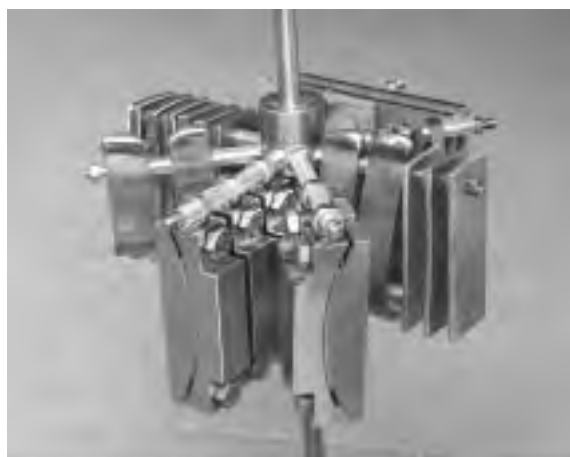
Fig.5 Corrosion monitoring system for SFIS
