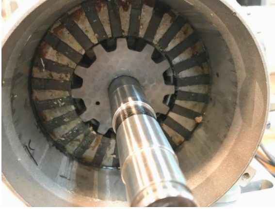
Figure 5.10. (a) Stator and Rotor Fitted Inside Frame.
