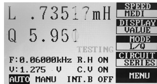
Figure 6.8. (c) Total winding inductance measurement using LCR meter.
