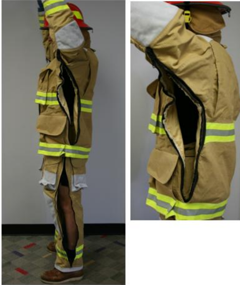
Figure 8-4. Active venting structural firefighter turnout prototype.
