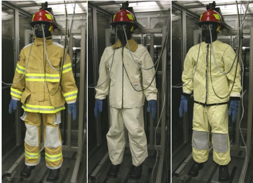
Figure 7-5. Outer shell, moisture barrier, and thermal liner garments tested for manikin THL on a sweating thermal manikin in a normal working condition scenario.
