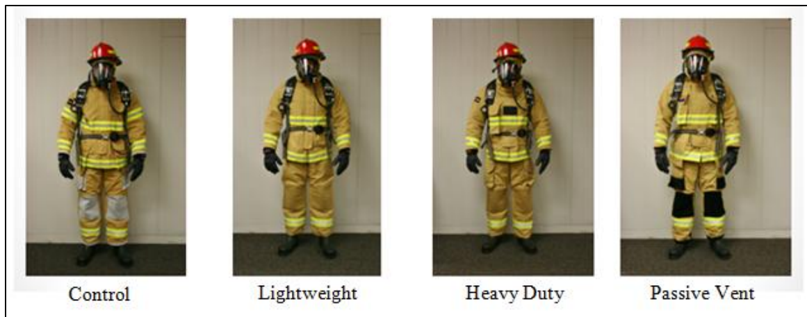
Figure 5-1. Suits tested with varying levels of bulk.
