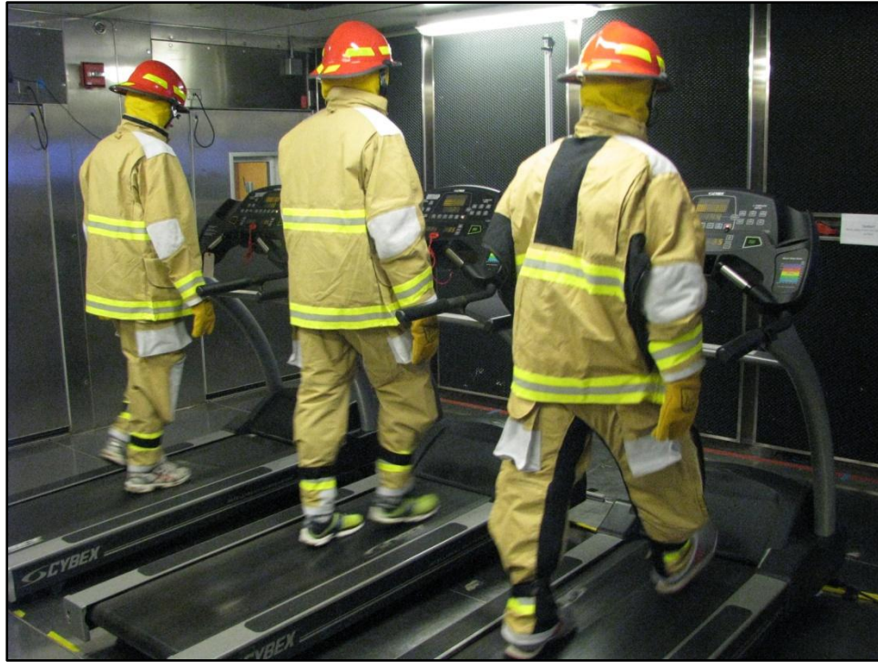
Figure 9-3. Wear trial subjects walking on treadmill at 3.5 mph at 3% incline.
