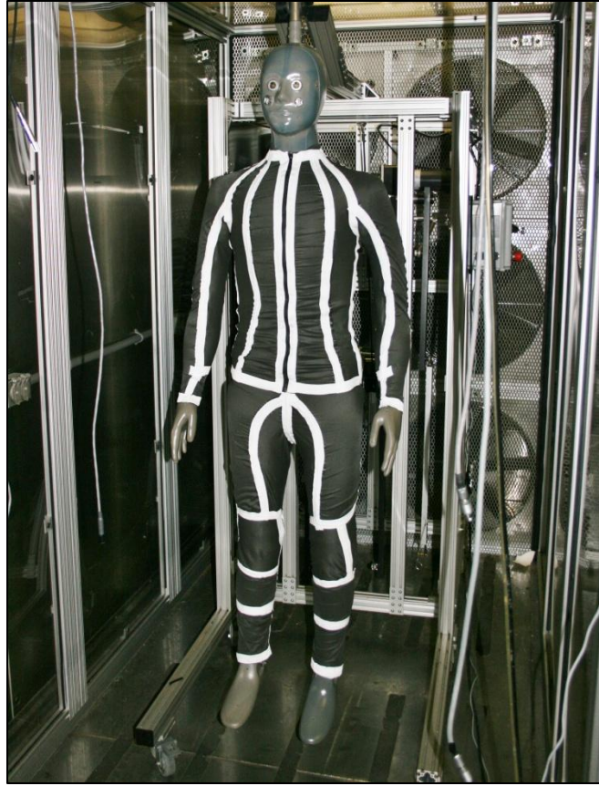
Figure 7-3. Tight fit moisture barrier garment dressed on sweating thermal manikin.
