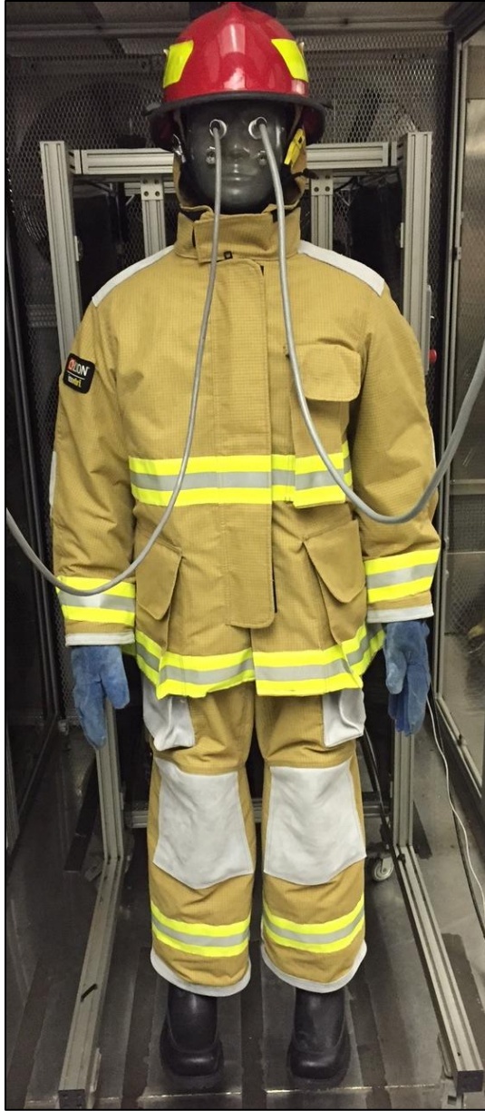
Figure 8-8. Control structural firefighter turnout tested in a vehicle extrication scenario on the sweating thermal manikin.
