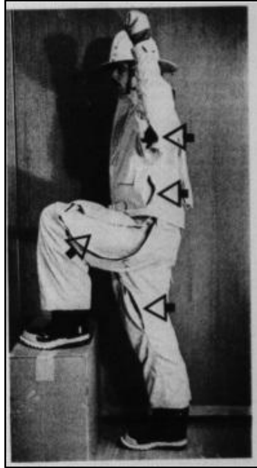
Figure 2-5. Bellows ventilation design of structural turnout gear (Reischl & Stransky, 1980a).
