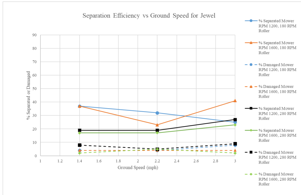
Figure 2.29: Separation efficiency and damage percentage of the harvesting aid for the Jewel variety at the three ground speeds for varying mower and roller rpm
