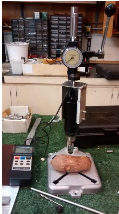
Figure 3.4: Modified version of the Halderson Periderm Shear Tester and Torquometer constructed at the BAE Research Shop, NCSU and integrated with the fruit pressure tester
