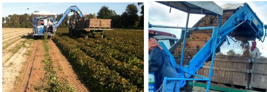
Figure 4.2: The field with the Beauregard roots being mechanically dug (left) and conveyed into the bins (right) by the STANDEN TSP 1900 sweetpotato mechanical digger during the 2016 harvesting season at Burch Farms, Faison NC
