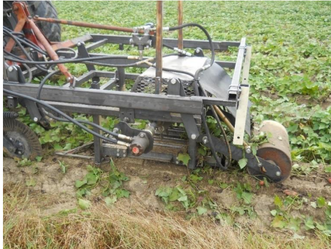
Figure 2.15: One-row vine puller-chopper prototype field testing during the 2014 harvesting season
