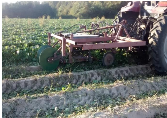
Figure 2.20: Field testing of the improved one-row vine puller-chopper harvesting aid hitched to a CASE 125 MAXXUM tractor in a field with the Covington sweetpotato variety, Burch Farms, NC
