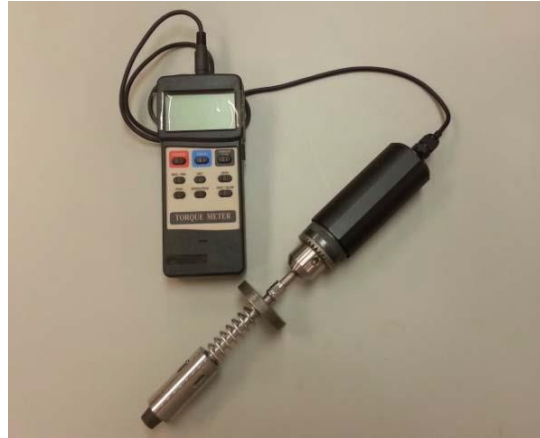
Figure 3.3: Digital torquometer and Halderson Shear Tester with spring loaded shaft for applying constant normal force (Hayes et al., 2014)
