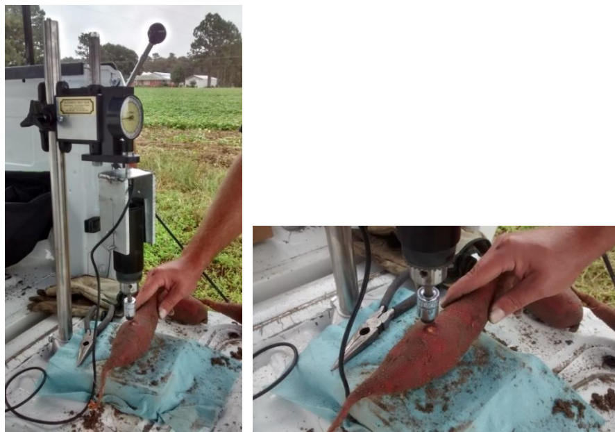
Figure 3.2: Modified version of the Halderson Periderm Shear Tester and Torquometer to measure the skin strength of the sweetpotato roots
