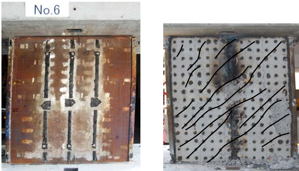
Figure 7. Steel plate and Concrete of post test inspection. (Case No. 6 (200 °C with membrane force))
