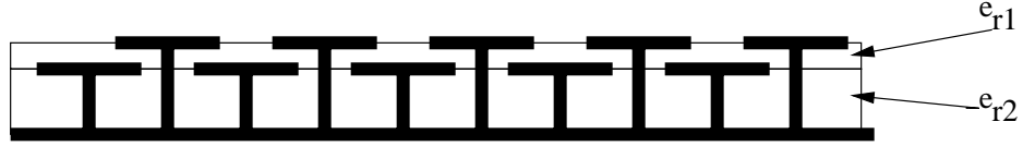
Figure 5.2: High Impedance ground plane with two layers of resonant elements.
