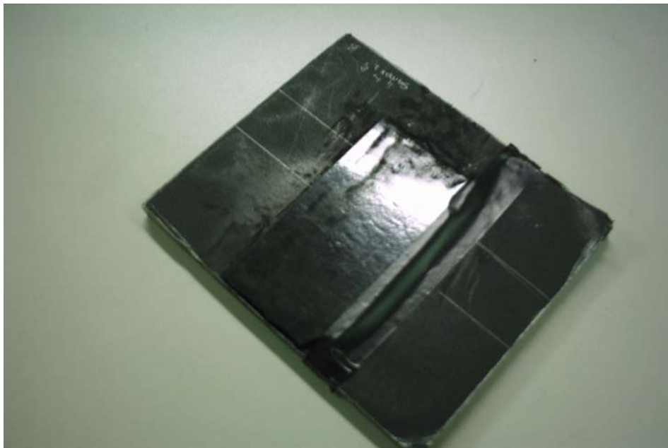
Figure 7-12 Seventy four Layer Specimen Prepared in Material Testing Station
