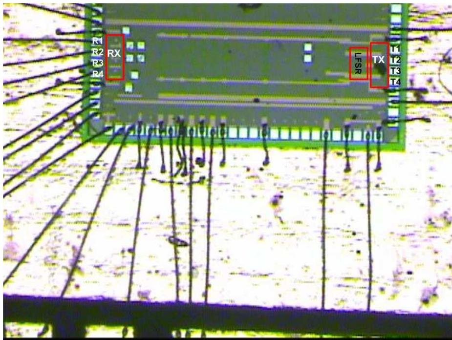
Figure 5.2: microphotograph of the fabricated IBM 0.13 \mu\text{m} CMOS test chip ( 3 \text{ mm} \times 1.5 \text{ mm} )
