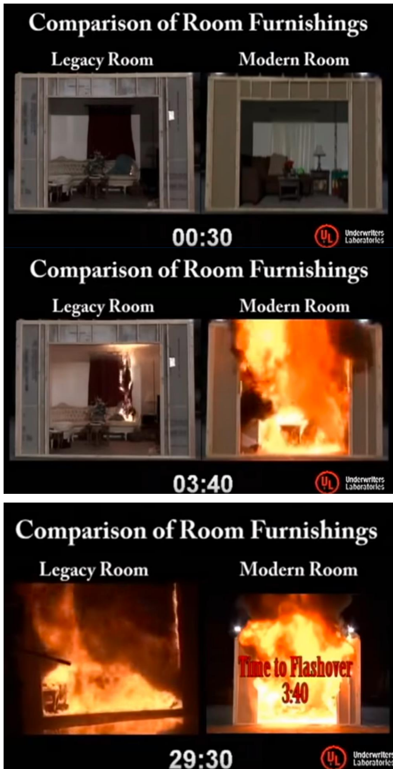
Figure 2: Images from a time-lapse demonstrating the time to reach flashover conditions of a room filled with legacy vs modern room furnishings [16]
