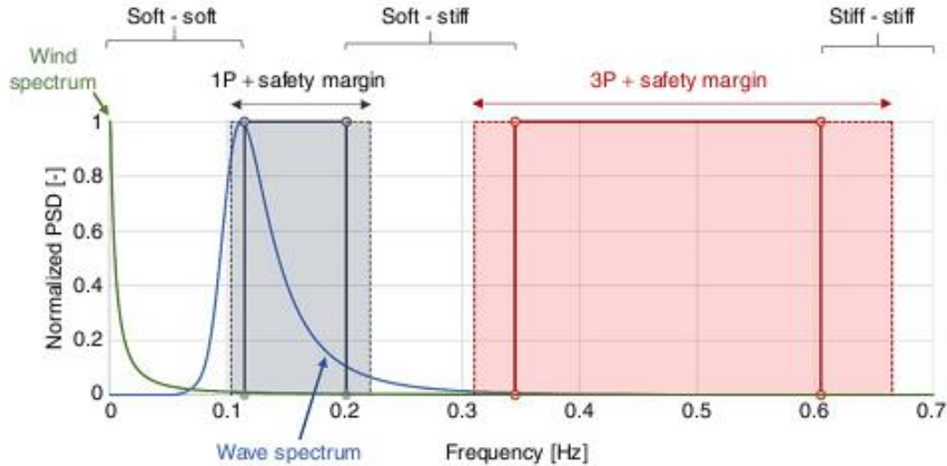
Figure 3.1. Normalized power spectral density (PSD) and frequency ranges of loads acting on offshore wind turbine system (Bhattacharya, 2019).
