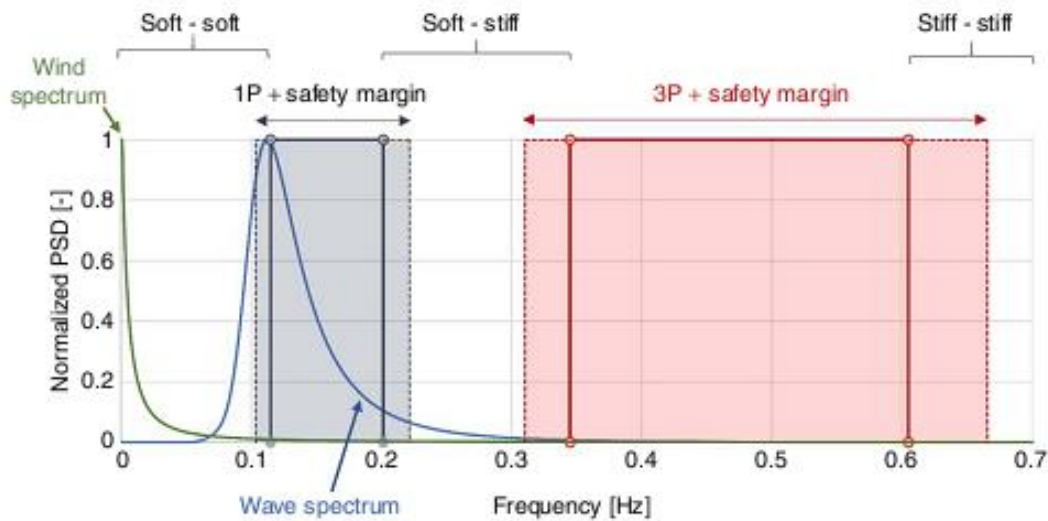
Figure 4.1. Normalized power spectral density (PSD) and frequency ranges of loads acting on offshore wind turbine system (Bhattacharya, 2019).
