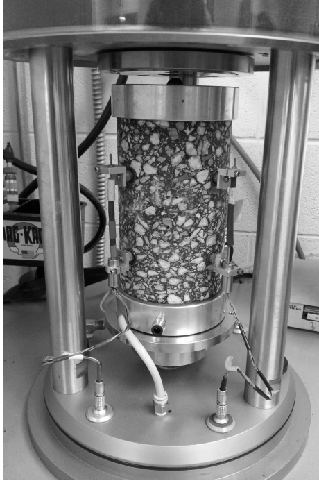
Figure 7.3: AMPT Test Specimen in the Test Device
