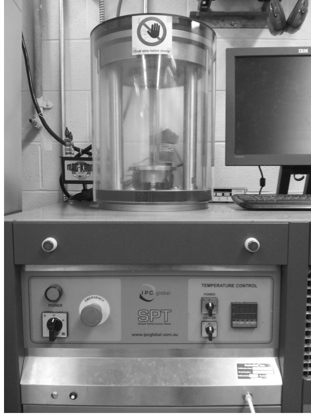
Figure 7.1: Asphalt Mixture Performance Tester (AMPT) Device
