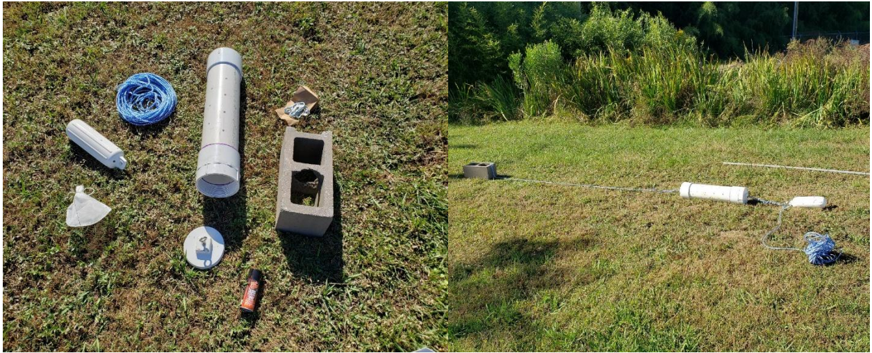
Figure C.4. Components for constructing PVC cylinders for seed submergence tests (left) and an assembled cylinder (right).
